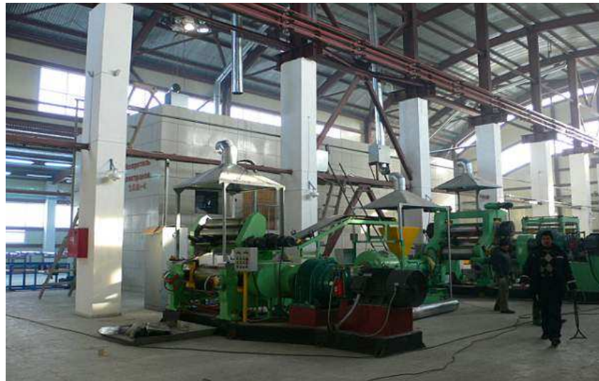
“Krovlen” roofing material production line
